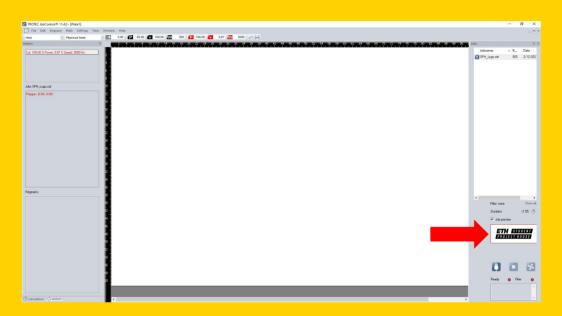
By pressing the small play button on the right, the job will be sent to the machine. The ventilation will turn on automatically and the job will start after 5 seconds.
