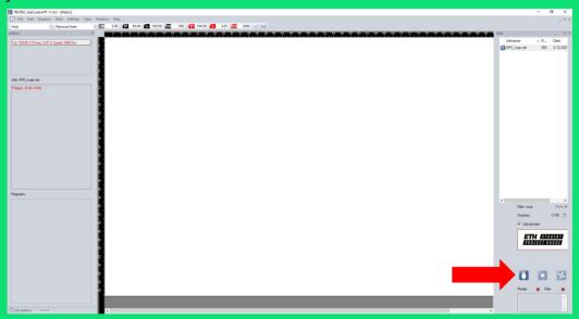
Select your job from the list on the right and drag it onto the virtual machine table left to it. The current laser position is indicated with the small crosshair. You can use it to position your job on the print bed.
